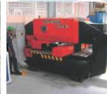
Turret Punch Machine: For punching of holes on reflector panel.
